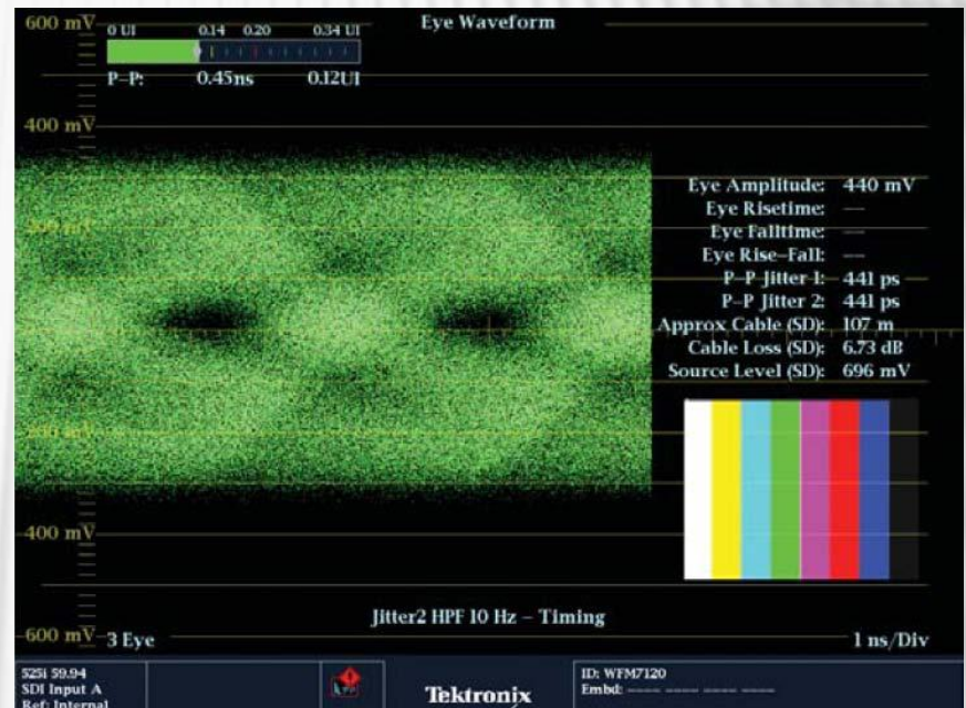
Figure 77. WFM7120 display of eye closure with long length of cable.
